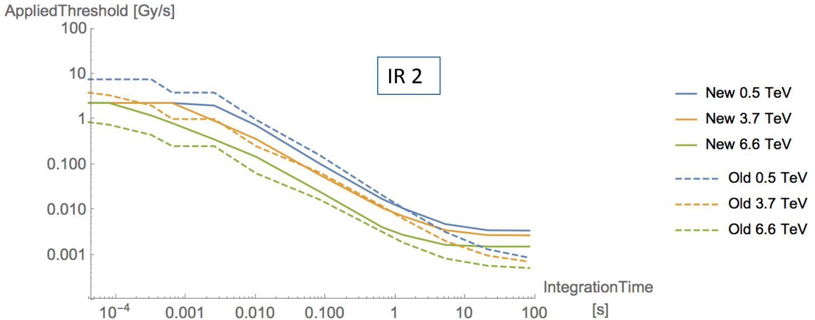
New thresholds at flattop comparable or higher than old ones.
