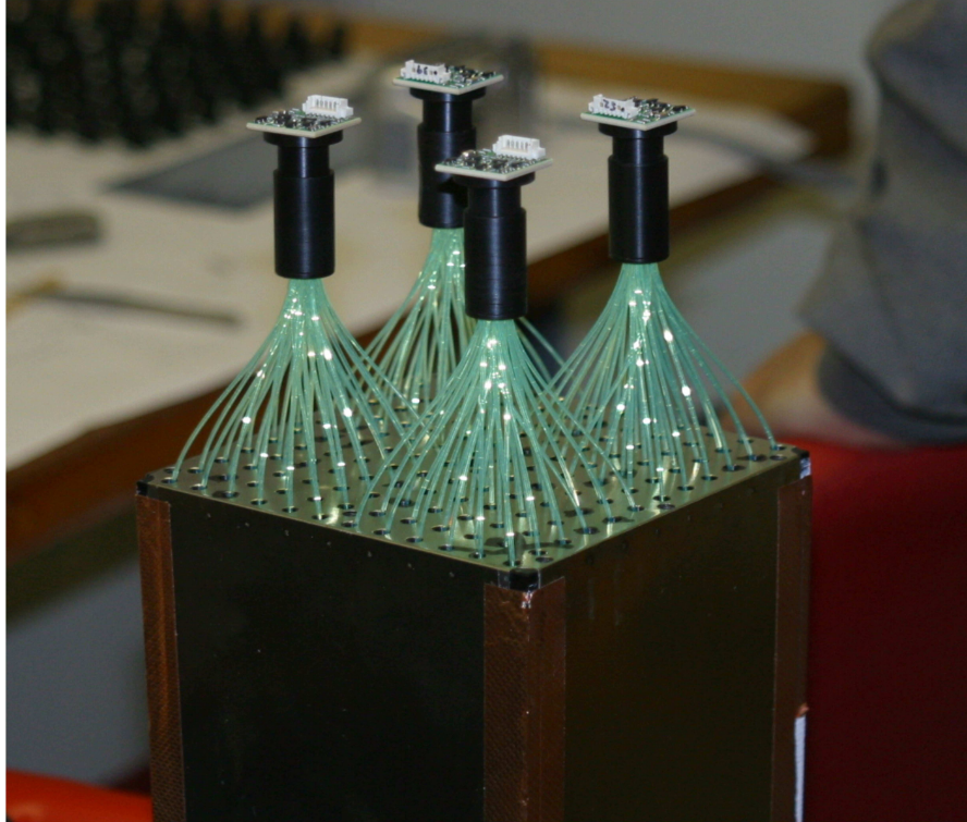
Figure 2.8: Fibre bundles with attached APD and preamplifier of four towers of an EMCal module.
