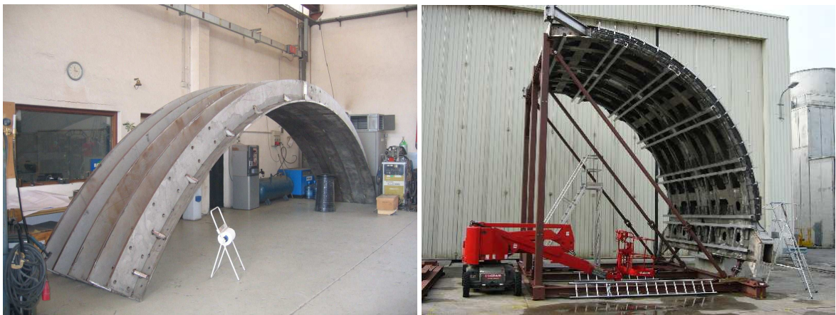
Figure 9.3: The CalFrame in the process of assembly (left) and fully assembled (right).
